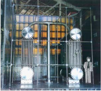
PCCS heat exchanger test
