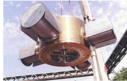
drywell to wetwell vacuum breaker test
